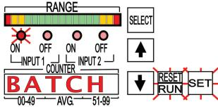
This procedure will establish the maximum amount of parts to be produced. Separate from the **TOTAL** counts.
