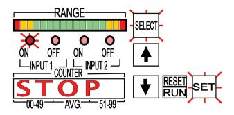
With STOP in the digital display, press SET then SELECT. Flashing display indicates first digit of low limit which may be adjusted by pressing ★ SELECT toggles to next digit. After low limit is completed, press SELECT again to adjust the first digit of the high limit. Repeat process above until high limits is complete. Recommended setting is 25 50 75. Limit values closer to 50 produce greater sensitivity. Pressing SELECT after setting limits will display TOTAL.
