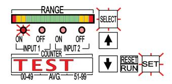
Control limit may be changed at anytime while ACE unit is monitoring production. Press SET then SELECT to alter first digit of low limit (follow procedure as outlined in "Setting Limits" section above). When new limits have been altered, press SET to resume production and control. Min/Max is the lowest and highest force value monitored during control mode. Press SELECT once to view limits then press SELECT again to view Min/Max.
