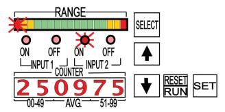
When an error occurs the unit stops production then displays the channel and exceeded limit value (bar graph indicates a low limit error when left red light is on, and a high limit error when the right red light is on).
