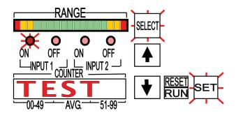
With **STOP** displayed, pressing RESET/RUN turns off all relays. **TEST** is now displayed. Manually start machine / press. ACE will now monitor up to 100/500 test parts before shutting off for operator input. Operator may press RESET/ RUN any time while in **TEST** to enter **LRN** mode. Following an 8 piece learn cycle, the ACE unit begins controlling production (a roaming green light appears in the bar graph). Use ♠ or ♣ to view ascending or descending counts.
